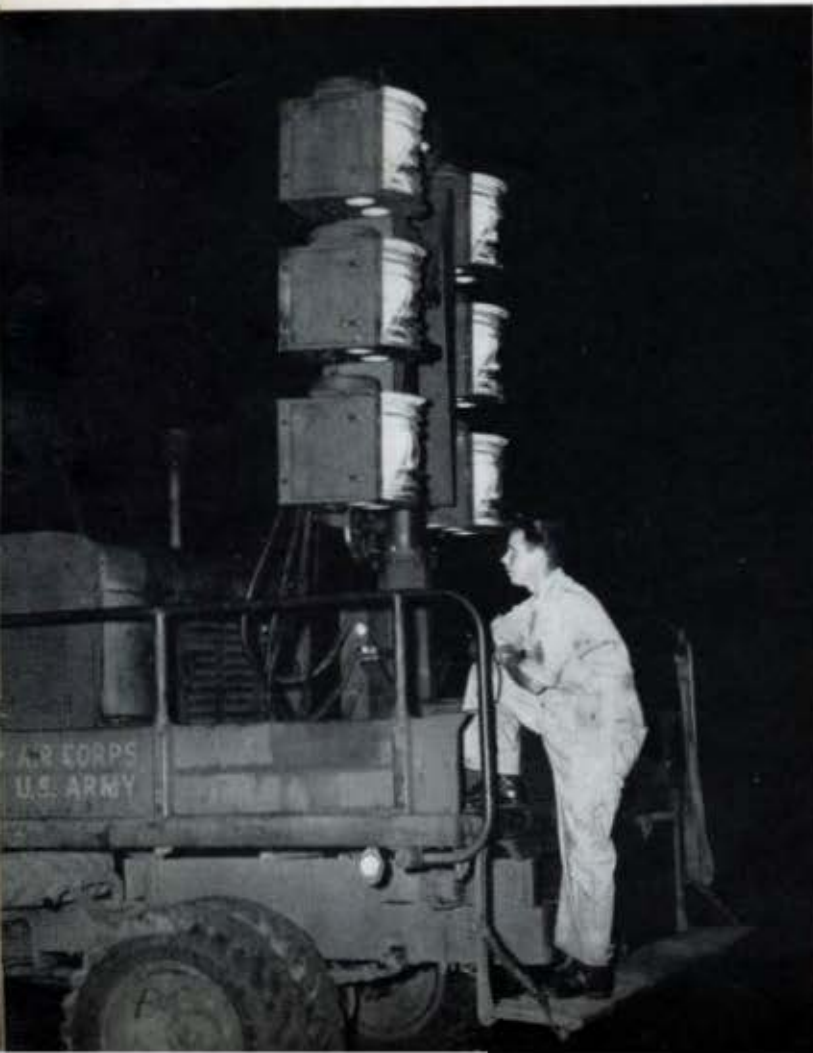
Portable landing lights.
