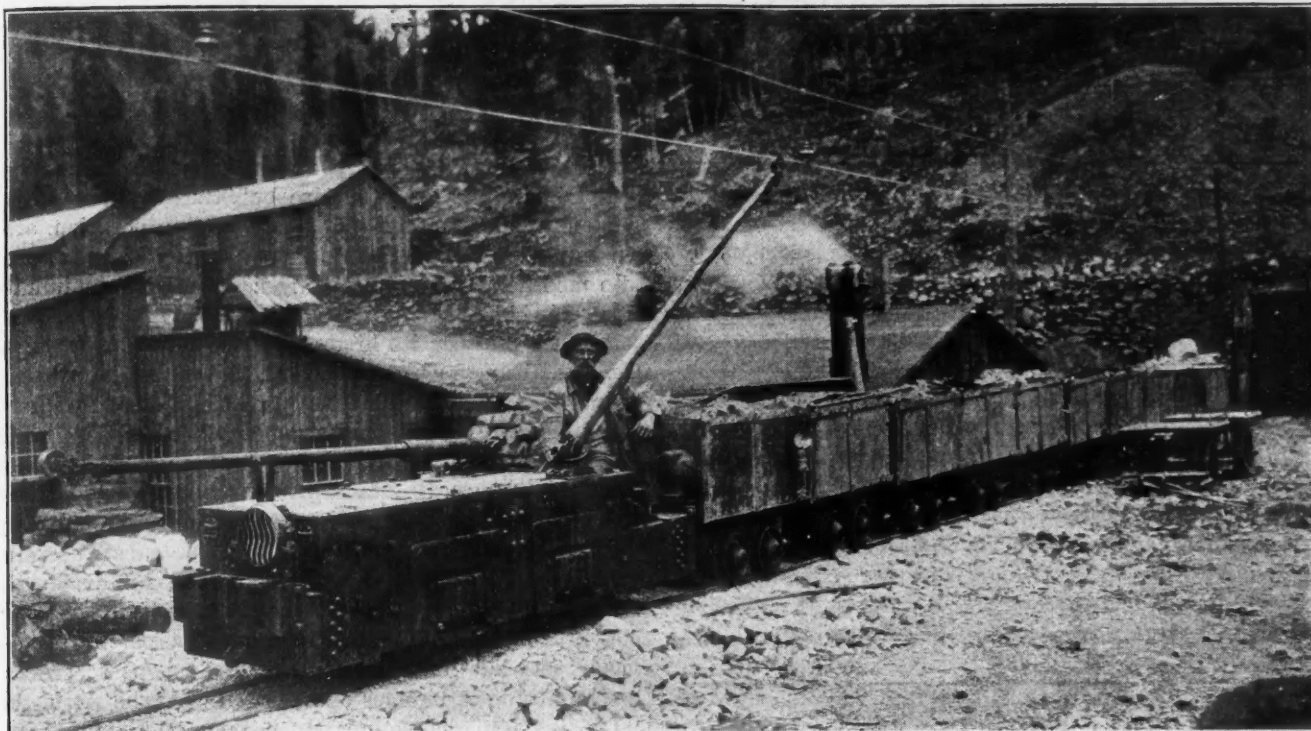
JEFFREY THREE-TON LOCOMOTIVE NOW USED FOR HAULAGE IN RAWLEY MINE
